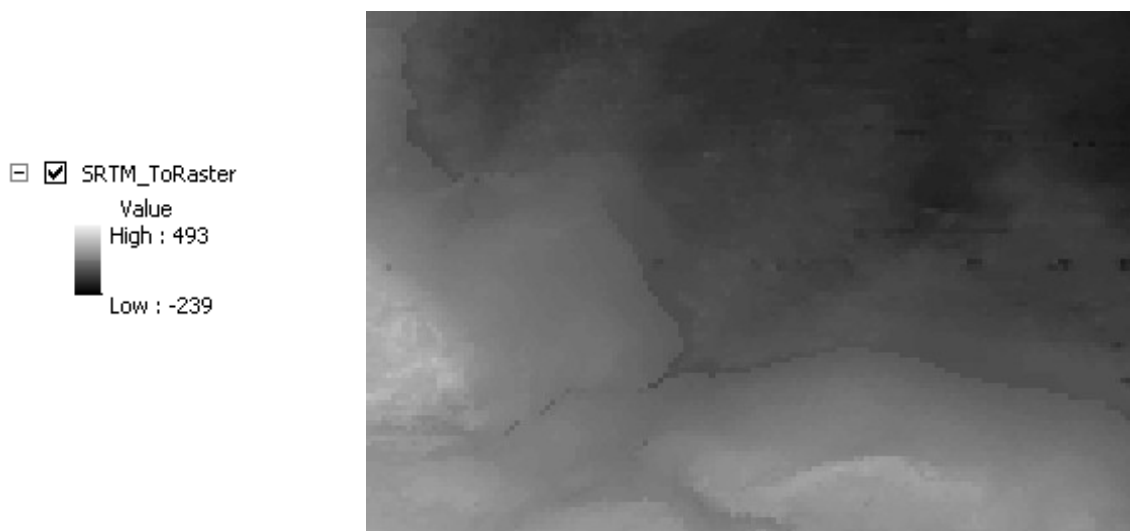
Raster surface derived from depth values of the point shapefile created in Step 3
