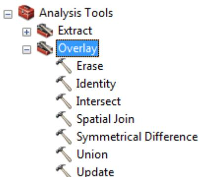
In this case, we wish to overlay glacier polygons with each interval created in Step 2 so that we can calculate the total glacial area that occurs within the given elevation values. This type of analysis can be achieved with the *Intersect* tool, which computes the geometric intersection of multiple features, as shown below.
