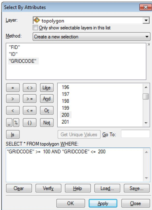
In the example shown here, we have selected all polygons that have an elevation value between 100 and 200 m above sea level.
