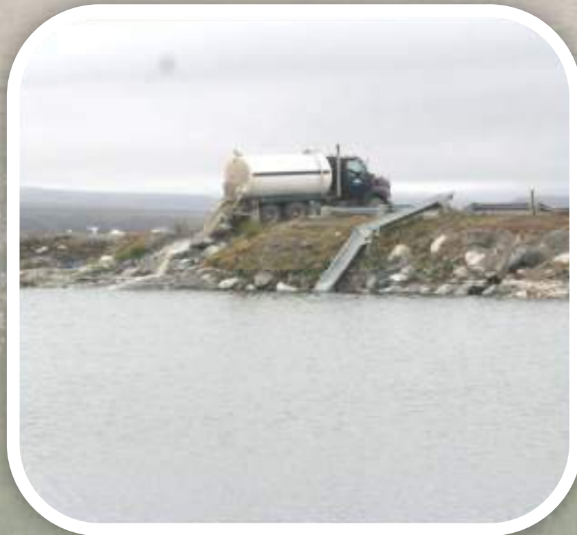
Figure 6. Sewage truck discharges in Ulukhaktok, NT
